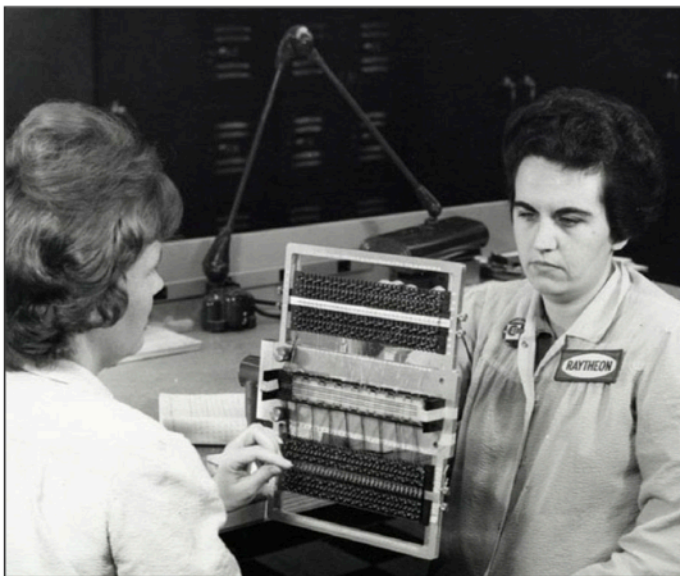
The memory was a complex mesh of wires and magnets. This was woven by a group of women who'd previously worked in watch-making factories.
